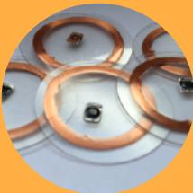
**RFID Tags Have a chip and a coil, the tag is passive which means there is NO Battery**
